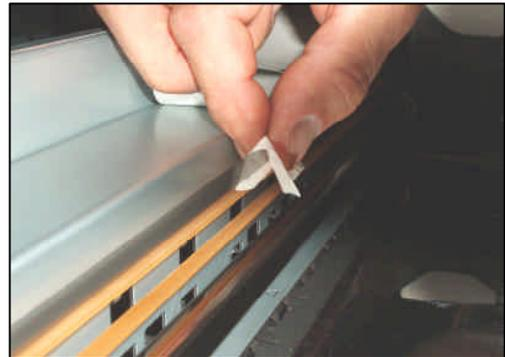
**Note: the Encoder Strip is actually CLEAR with small marks on it. Be careful to NOT scratch it or the sensor will not read it correctly.**
